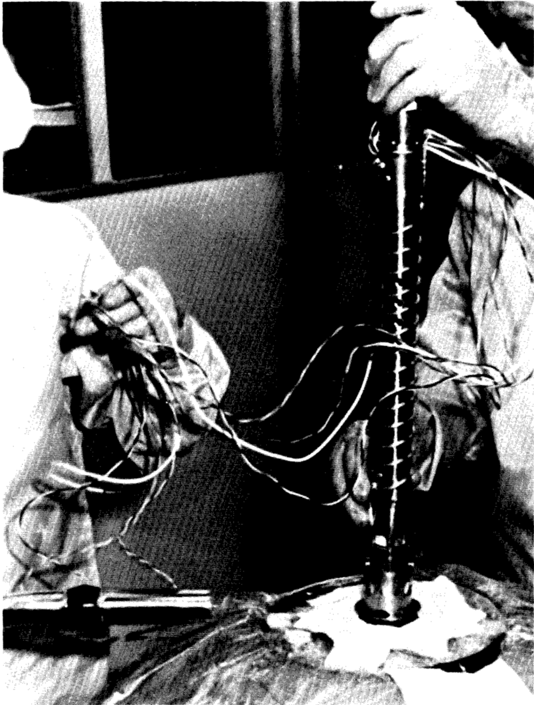
Figure C4-31.- Inserting fan and heater probe.
