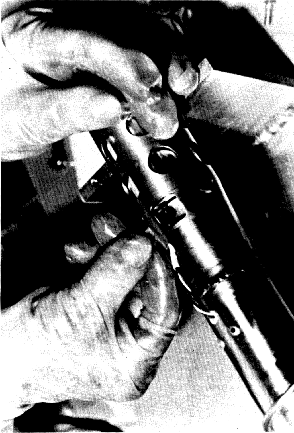
Figure C4-13.- Inserted copper band to retain motor wires.
