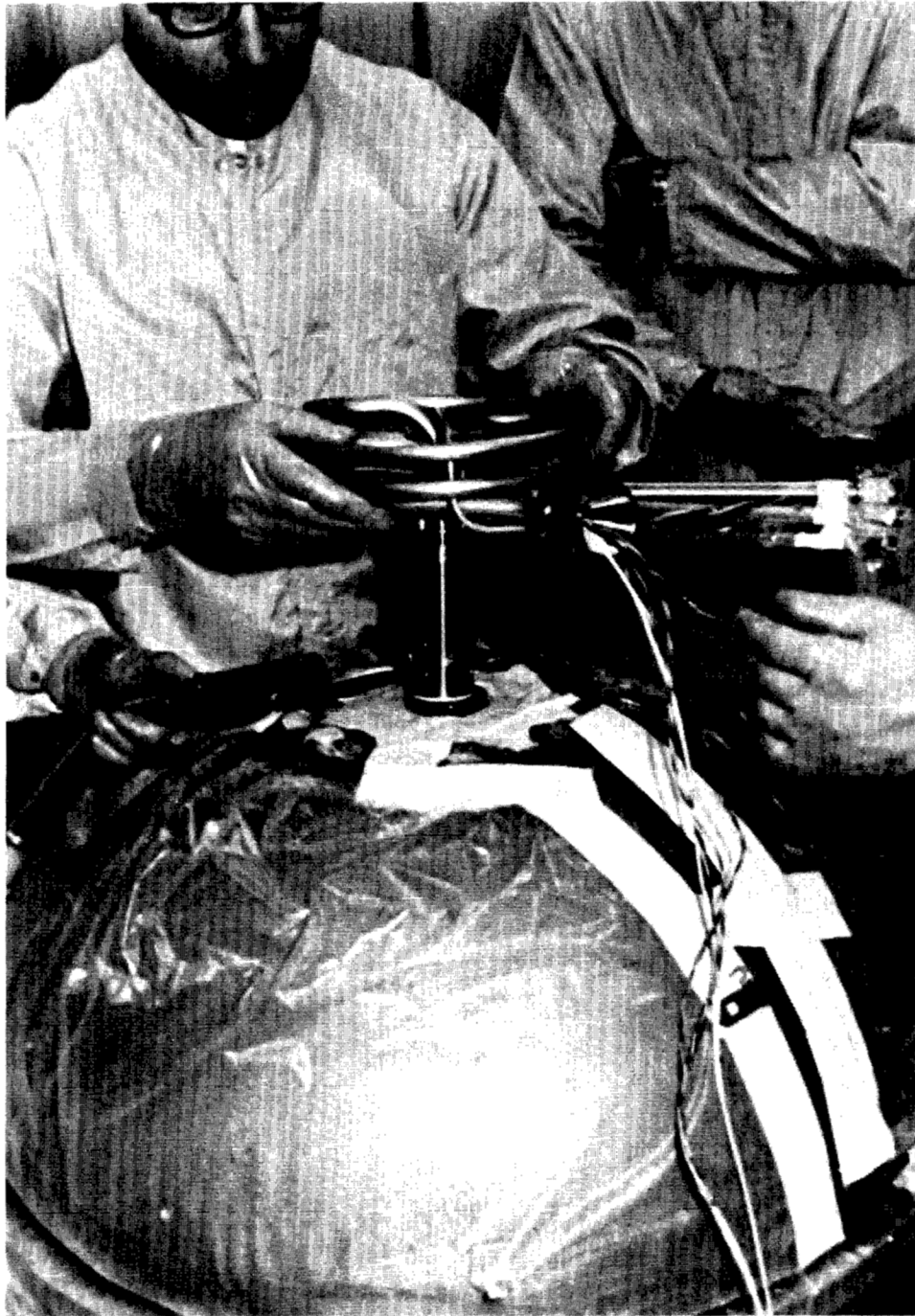
Figure C4-44.- Lowering quantity probe assembly into tank.
